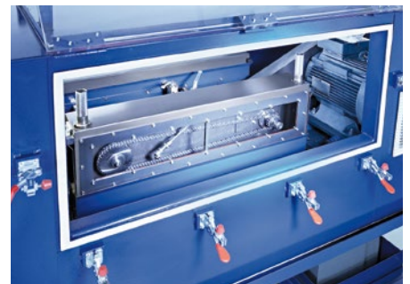
Testing of chain wear elongation behaviour on more than 20 test rigs
